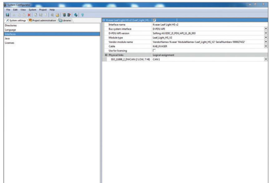
> Check that the connection status „Connected“ is displayed and that the correct serial number is displayed for the diagnostic interface.
