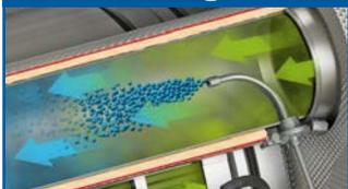
The reduction agent in the AdBlue® tank ⑤ is injected into the exhaust system according to the NO<sub>x</sub> concentration measured by the system electronics. It is then converted to ammonia in the mixing section that follows.
