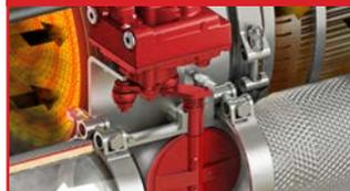
The exhaust gas temperature is raised by means of the eFlow controller. For this purpose, the exhaust backpressure is adjusted to a constant value. Within a fraction of a second, the control angle of the eFlow controller is adjusted as a function the exhaust mass flow and exhaust-gas temperature. At high temperatures and high mass flows, the eFlow controller is fully open.
